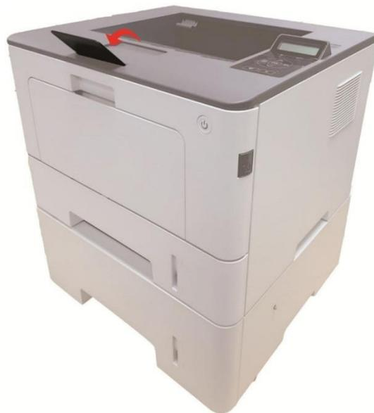
**Note:** • If more than 550 pieces of paper (80g/m<sup>2</sup>) are put inside the optional tray at one time, it will lead to paper jam or paper feed failure.
