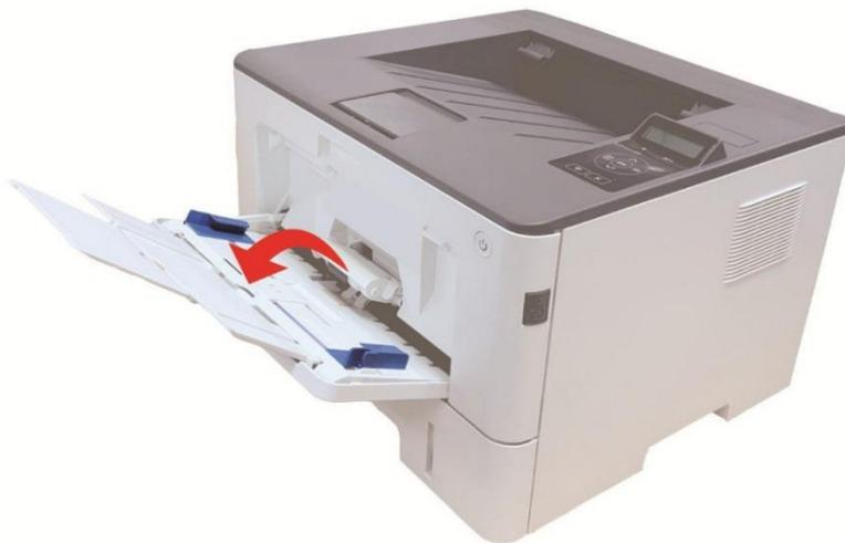
2. Slide the paper guide of the multipurpose feed tray to match both sides of the paper. Do not apply excessive force; otherwise, paper jamming or tilting may occur.
