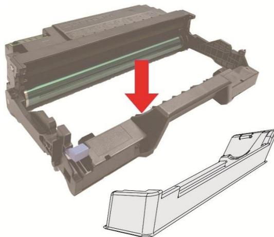
5. Install the drum component along the inner track to finish installing toner cartridge.
