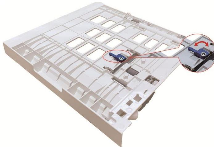
4. Install the duplex unit in the printer.
