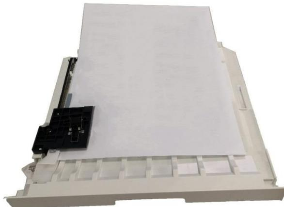
3. If the paper does not come out along with the duplex unit, open the tray and remove the jammed paper directly from the bottom.
