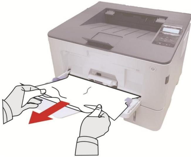
2. After removing the jammed paper, reload paper into the multi-purpose tray; press the front cover button to open and close the front cover, and the printer will resume printing.
