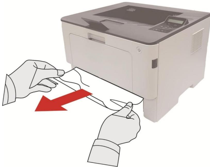
3. After removing the jammed paper, reinsert the automatic tray into the printer; press the front cover button to open and close the front cover, and the printer will resume printing automatically.
