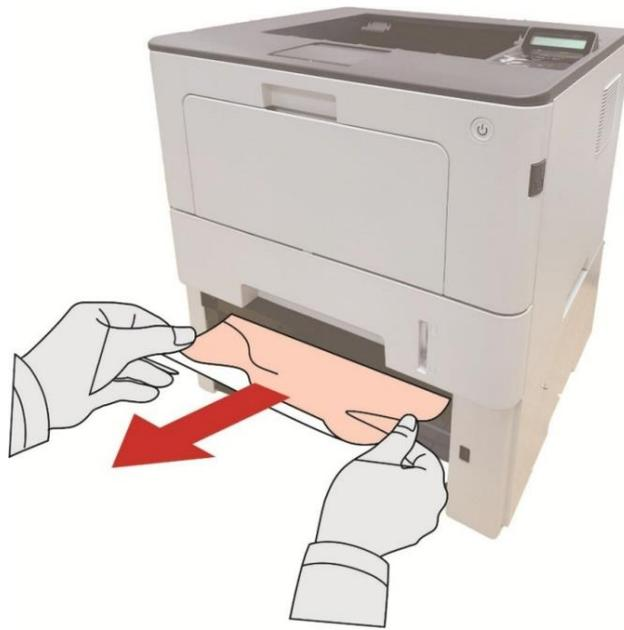
3. After the jammed paper is removed, install the Auto Feed Tray into the printer. Open and close the front cover. The printer will automatically reprint
