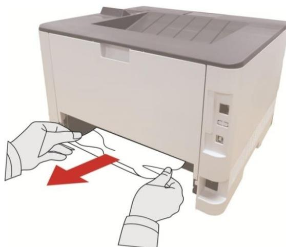
4. After taking papers jammed out, install the duplex unit back and inspect other parts to the product. If it can be ensured that there are no jammed papers, open and close the front cover and then the printer will recover printing automatically.
