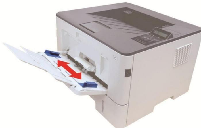
3. Unfold the stack of paper for feeding to avoid jamming or feeding error, place the side of paper to be printed upwards into the automatic feed tray. The multipurpose feed tray can hold up to 60 pieces of 80g/m<sup>2</sup> paper.
