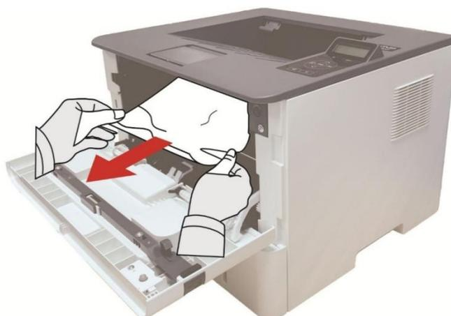
7. After taking out papers jammed, install the laser toner cartridge again and close the front cover, then the printer will recover printing.
