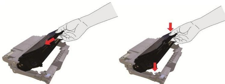
7. Take the drum component with toner cartridge installed and install it inside the printer along the inner track of printer to finish installing.
