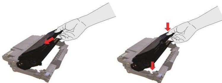
6. Take the drum component with toner cartridge installed and install it inside the printer along the inner track of printer to finish installing.
