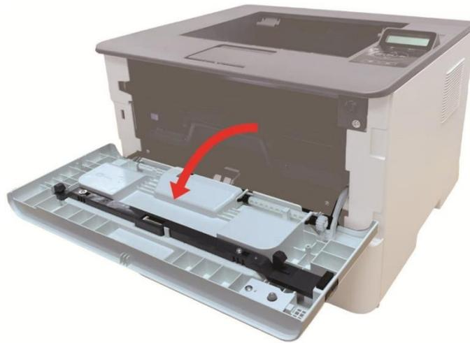
5. Take the laser toner cartridge out along the track. (For the purpose of preventing printing quality from affecting by the exposure of photosensitive drum, please put the laser toner cartridge inside the protection bag or wrap it with thick paper).
