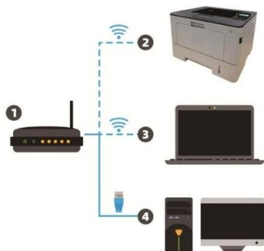
Basic structure mode: connecting to a wireless device via router
