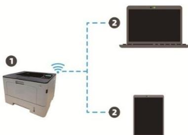
Wi-Fi Direct mode: wireless client is connecting to a printer with Wi-Fi function
