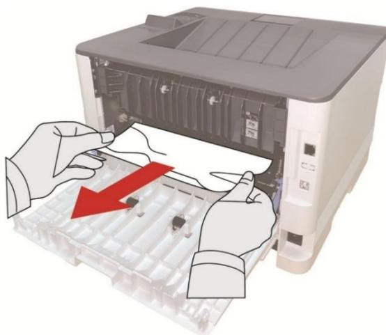
4. After taking papers jammed out, close the back cover and open the front cover and then the printer will recover printing.
