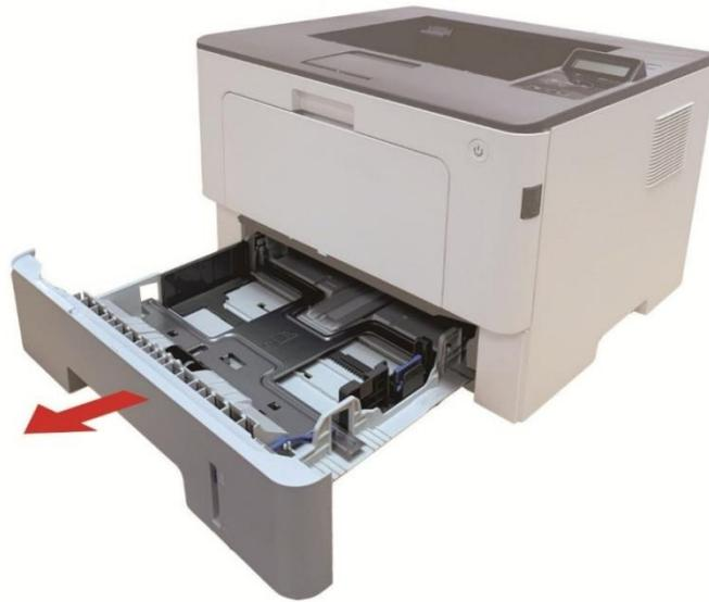
2. Slide the clip of extended tray of auto feed tray, paper length deflector and paper width deflector to the slot suitable for paper size, in order to match paper length and width.
