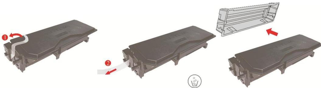
6. Install the drum component along the inner track to finish installing toner cartridge.
