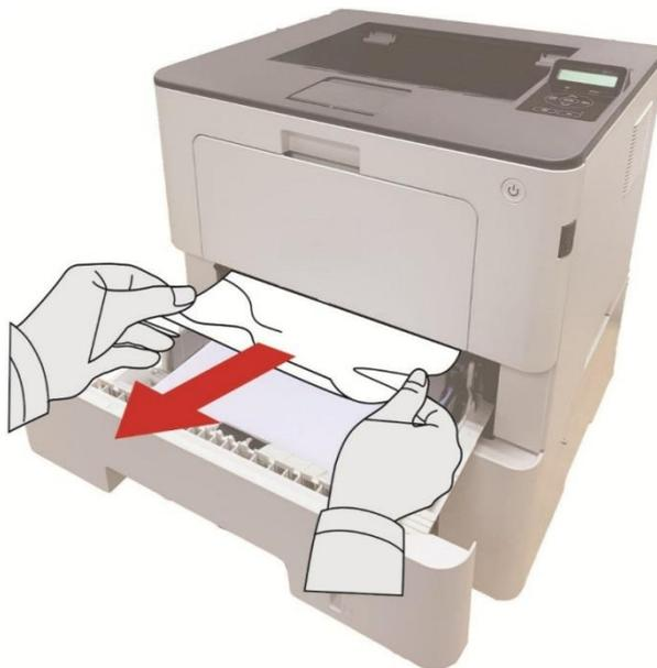
3. After removing the jammed paper, reinsert the automatic tray into the printer, and the printer will resume printing automatically.
